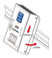
**Step 3:** Check whether the DIN-rail is tightly on the track.
