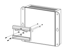
**Step 2:** Lightly insert the bottom of DIN-rail into the track.
